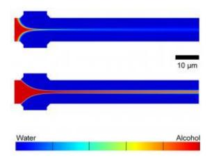
Computer simulations showing the mixing of water and isopropyl alcohol in a COMMAND microfluidic device. The alcohol, which would be mixed with dissolved phospolipids in operation, flows from the left to the right via the center inlet and is focused by water flowing in from the top and bottom inlets. Adjusting flow rates gives a tightly focused stream (top) or broader (bottom), controling liposome size. Credit: NIST
