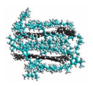
Two graphene molecules (dark grey) are caged by sidegroups (blue) attached to each graphene sheet. The sidegroups help prevent the graphene sheets from stacking, as they are prone to do. Credit: Image by Liang-shi Li
