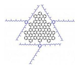
This is a 2-D view of a graphene sheet (black) and attached sidegroups (blue) that IU Bloomington chemist Liang-shi Li and his collaborators devised. In reality, each sidegroup rotates 90 degrees or so out of graphene's plane. The three blue, tail-like hydrocarbons of each sidegroup have great freedom of movement, but two are likely to hover over the graphene, making it very unlikely that one graphene sheet will touch another. Credit: Image by Liang-shi Li
