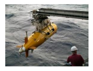
This is the launch of the British robot submarine Autosub6000. Credit: NOC
