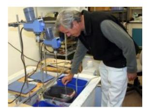
Bart Chadwick, head of the Environmental Sciences Branch of Space and Naval Warfare Systems Center Pacific, checks conditions in laboratory microbial fuel cells. The fuel cells may revolutionize naval energy use by converting decomposed marine organisms into electrical energy, offering a clean, efficient and reliable alternative to batteries and other environmentally harmful fuels. Credit: US Navy photo by John F. Williams
