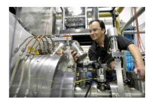
Engineer Richard Vondrasek installs a new turbo pump on the Californium Rare Isotope Breeder Upgrade (CARIBU). CARIBU reached world record efficiencies for ionization efficiency of solids.
