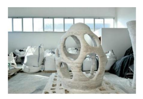
(PhysOrg.com) -- An Italian inventor, Enrico Dini, chairman of the company Monolite UK Ltd, has developed a huge three-dimensional printer called D-Shape that can print entire buildings out of sand and an inorganic binder. The printer works by spraying a thin layer of sand followed by a layer of magnesium-based binder from hundreds of nozzles on its underside. The glue turns the sand to solid stone, which is built up layer by layer from the bottom up to form a sculpture, or a sandstone building.
