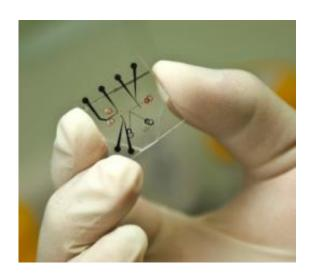
A single unit of the new desalination device, fabricated on a layer of silicone. In the Y-shaped channel (in red), seawater enters from the right, and fresh water leaves through the lower channel at left, while concentrated brine leaves through the upper channel. Photo: Patrick Gillooly
