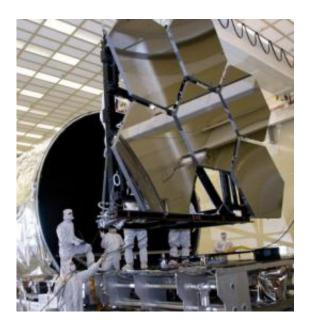
The mirrors were cryogenically tested by Ball Aerospace at the X-ray and Cryogenic Facility, at Marshall Space Flight Center. Credit: NASA/MSFC/Emmett Givens
