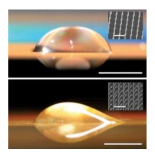
A symmetrical droplet (top) forms on a surface with straight nano-pillars, while on a surface with bent pillars (bottom) the droplet is asymmetrical, extending out only to the right. Inset images are micrographs of the surface structure. Images: Kuang-Han Chu, Rong Xiao and Evelyn N. Wang
