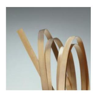
This is high temperature superconducting wire developed by UH researcher Venkat Selvmanickam. Credit: Courtesy of the University of Houston
