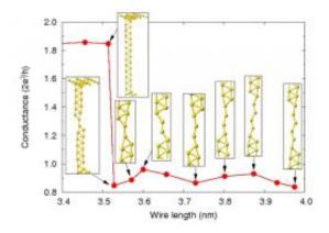
A quantum-mechanics-based simulation demonstrates how a new NIST instrument can delicately pull a chain of atoms apart. The chart records quantum jumps in conductivity as a gold contact is stretched 0.6 nanometer. The junction transitions from a 2-dimensional structure to a one-dimensional single-atom chain, with a corresponding drop in conductivity. Following the last point, at a wire length of 3.97 nm, the chain broke. Credit: Tavazza, NIST
