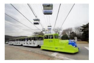
The Online Electric Vehicle (OLEV), towing three carriages, runs along a blue line under which power strips are buried for recharging, at an amusement park in Gwacheon, south of Seoul. S.Korean researchers launched an environmentally-friendly public transport system using a "recharging road" -- with a vehicle sucking power magnetically from buried electric strips.
