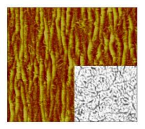
This atomic-force microscopy image shows wrinkling in a single-wall carbon nanotube membrane; the inset shows an optical reflection micrograph of the membrane without any strain. The random arrangement of the nanotubes shown in the inset creates conductivity, but wrinkling can disrupt that. Each image is 40 micrometers in width. Credit: NIST
