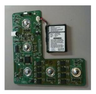
MIT engineers have designed this wearable ECG monitor that runs on very little power and could replace cumbersome devices now used to monitor heart patients. Photo: Eric Winokur
