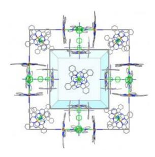
The crystal structure of the nanoporous crystal showing the "molecular wall-tie" ligands (green) binding between the iron centres.
