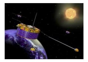
ESA's mission Cluster consists of four identical spacecraft flying in formation between 19 000 and 119 000 km above the Earth. They study the interaction between the solar wind and Earth's magnetosphere, or the Sun-Earth connection in 3-D. Credit: ESA
