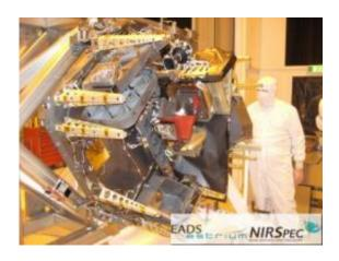
The NIRSpec Engineering Test Unit was provided by the European Space Agency, with EADS-Astrium GmbH as Prime Contractor. NIRSpec will be the principal spectrographic instrument on board the Webb telescope. Credit: EADS Astrium
