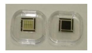
The PV cell prototyped at the Kyoto Institute of Technology by adding cobalt to a p-type GaN thin film and laminating an n-type material (right). The cell with an absorbing layer measures 10 x 10mm. The surrounding thin rectangular patterns are electrodes. And the p-type GaN thin film without cobalt (left). Image via: Tech on.
