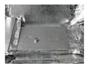
A pressure sensor inside the vacuum insulation panel constantly checks whether the vacuum is still present. Credit: Fraunhofer IMS
