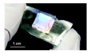
The PZT ribbons covering this minuscule rubber chip have the capacity to harness energy generated from body motions. [Credit: Nano Letters]
