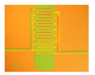
Princeton researchers have developed a new way to manufacture electronic devices made of plastic, employing a process that allows the materials to be formed into useful shapes while maintaining their ability to conduct electricity. In the plastic transistor pictured here, the plastic is molded into interdigitated electrodes (orange) allowing current flow to and from the active channel (green). (Image: Loo Research Group)
