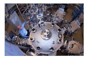
NREL engineer John Scharf sits at the hub of the robot in the Process Development and Integration Laboratory that works with solar cells using Copper Indium Gallium diSelenide (CIGS). The NREL researchers like to equate the robot's capabilities to a jukebox, shuffling in and out tools to grow and analyze solar cells. Credit: Pat Corkery
