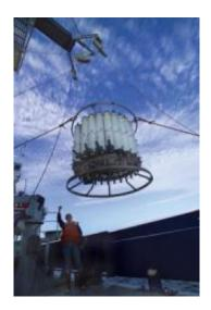
CalCOFI CTD seawater sampling such as this is augmented by data from satellites, research buoys and robotic gliders to track the physical and biological response to El Niño. Credit: Scripps Institution of Oceanography, UC San Diego
