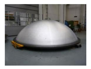
The second single-piece 5.5 meter diameter full-scale spun form dome was manufactured from a flat plate "blank" made from two pieces of aluminum lithium 2195 plate which were friction stir welded together. Image credit: MT Aerospace
