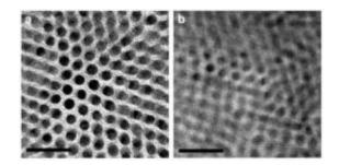
These transmission electron microscope images show (a) the original nanorod array of cadmium sulfide and (b) a composite made from cadmium sulfide and the chalcogenide copper sulfide. In the composite, nanoparticle ordering is maintained but spacing between the particles decreases. Credit: Delia Milliron, Berkeley Lab
