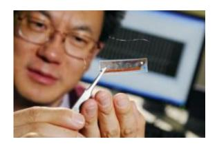
Georgia Tech professor Zhong Lin Wang holds an improved nanogenerator containing 700 rows of nanowire arrays. The generator was used to power nanometer-scale sensors. Credit: Photo: Gary Meek
