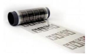
RFID tags printed through a new roll-to-roll process could replace bar codes and make checking out of a store a snap. Credit: Gyou-Jin Cho/Sunchon National University
