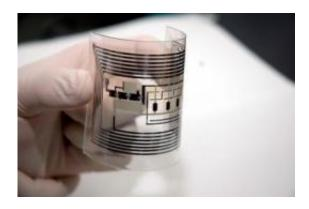
RFID tags printed through a new roll-to-roll process could replace bar codes and make checking out of a store a snap. Credit: Gyou-Jin Cho/Sunchon National University
