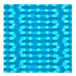
Polymer molecules can be deposited onto computer chips where they arrange themselves into small-scale patterns like the one shown here. Credit: Yeon Sik Jung and Joel Yang.
