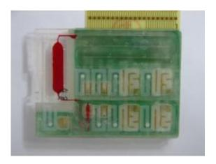
With the disposable cartridge, all diagnosis steps take place automatically, from collection of the specimen to data analysis. Credit: Fraunhofer IBMT
