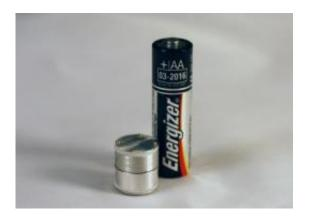
Miniature generators developed at U-M's Engineering Research Center for Wireless Integrated Microsystems run on the random vibrations all around us. Credit: Tzeno Galchev
