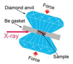
Diamond anvil cell used for high-pressure experiments.
