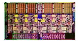
Code-named "Gulftown" the 32nm, six-core i7-980X is based on the current Westmere architecture and will be labeled as the i7x "Extreme Edition". It will be the first dual-socket, six-core processor from Intel.
