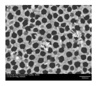
This scanning electron micrograph was obtained from a zinc oxide-coated nanoporous alumina membrane. Credit: Dr. Roger Narayan, North Carolina State University
