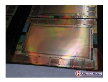
Here the fabrication of thin film transistor arrays can be seen on a flexible plastic material.
