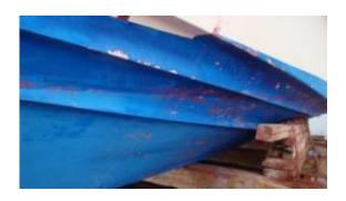
Organisms live off of the decomposing epoxy and polyurethane plastic paint used to seal the hull of this ship. Credit: Katsuhiko Saido
