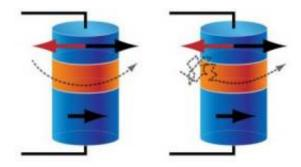
This is a schematic of data storage in (left) converntional magnetic memory and (right) thermally assisted memory. Credit: Illustration: Alan Stonebraker, APS
