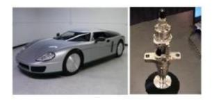
The new fuel-injection system is placed into this sports car which weighs approximately the same as the Toyota Prius hybrid and has similar aerodynamics. The new fuel injection system gets better gas mileage than the Prius hybrid. Credit: Transonic Combustion
