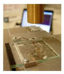
The Cottonscope instrument directly measures the maturity of cotton fibres within 25 seconds. (CSIRO)
