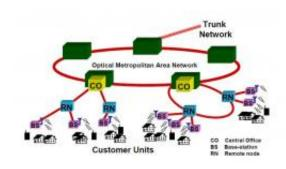
A mm-wave Fi-Wi network. An optical fiber backbone (red) provides broadband connections between the central offices and antenna base stations. Then, the base stations wirelessly transmit 5-mm-wave (60 GHz) signals to customers. Within buildings and homes, the short-range wireless signals can provide high-speed connectivity (faster than 1 Gb/s) for a variety of wireless, high-bandwidth communication devices. Credit: Lim, et al.
