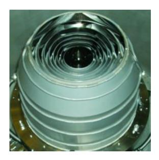
Media Lario's extreme ultraviolet (EUV) collector mirrors for semiconductor lithography are based on the original investment in the technologies and competences needed to produce the optical mirrors for ESA's XMM-Newton spacecraft. The EUV collector will be used in the production of the next-generation of faster and smaller integrated semiconductor circuits. Credits: Media Lario Technologies
