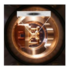
The picture shows the team's experimental apparatus comprising of the ion trap inside the vacuum chamber. The inset shows schematically the single ion (red) in the Bose-Einstein condensate (dark grey).
