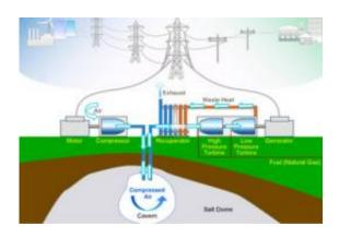
Compressors use off-peak electricity to fill the cavern with compressed air. For peak demand, the compressed air is withdrawn from the cavern and used to power a wind turbine. Credit: Ridge Energy Storage & Grid Services LP
