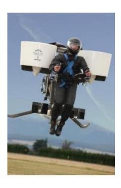
The Martin jetpack can fly for 30 minutes on a five-gallon tank of gas, reaching a top speed of 60 mph. Credit: Martin Aircraft Company.
