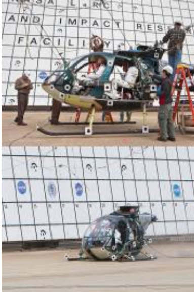
The MD-500 before and after the drop test. Credit: NASA/Sean Smith
