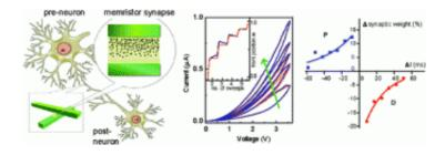
A memristor is a two-terminal electronic device whose conductance can be precisely modulated by charge or flux through it. Image credit: Nano Letters, DOI:10.1021/nl904092h
