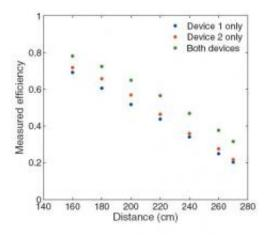
As the figure shows, the overall power transfer efficiency of the wireless system can be increased by powering multiple devices simultaneously, rather than each device individually. Using more than one device increases the coupling resonance. Reprinted with permission from Kurs, et al. Copyright 2010, American Institute of Physics.
