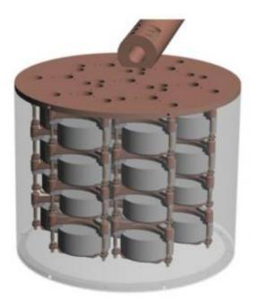
Conceptual drawing of the germanium-76 detector array.
