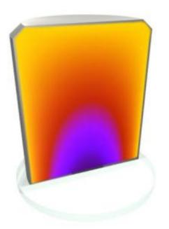
Section view of a germanium detector showing its electrical potential. The point contact is on the bottom and the electrical potential drops off to the outer wall of the cylinder.
