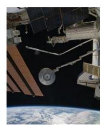
In this image provided by NASA the Tranquility module is transferred late Thursday evening Feb. 11, 2010 from its stowage position in space shuttle Endeavour's payload bay in the grasp of the station's Canadarm2 to position it on the port side of the Unity node of the International Space Station. Tranquility was locked in place with 16 remotely-controlled bolts. Earth's horizon and the blackness of space provide the backdrop for the scene. (AP Photo/NASA)
