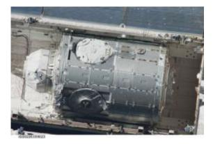
Node-3 and Cupola in the cargo bay of Space Shuttle Endeavour. Photograph was taken during the 'flip' manoeuvre that exposed Shuttle's heat shield for inspection from the ISS. Credits: NASA
