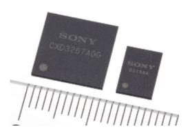
Sony's transceiver IC is the core of TransferJet short-range wireless technology.
